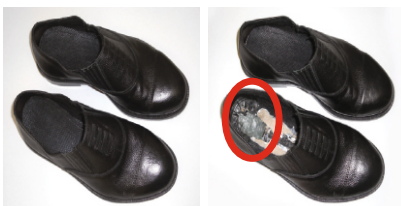
Fig. 6. Dangerous inclusion in heel
